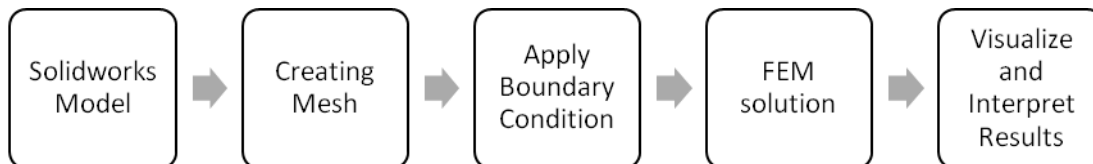
Figure 10 Finite Element Method Procedure
